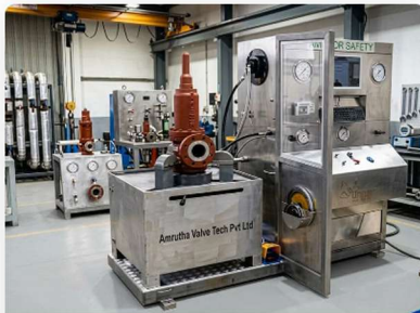
Safety Valve Test Stand
