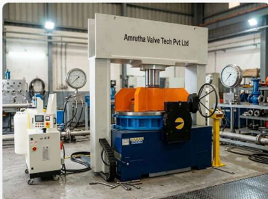
Butterfly Valve Test Rig
